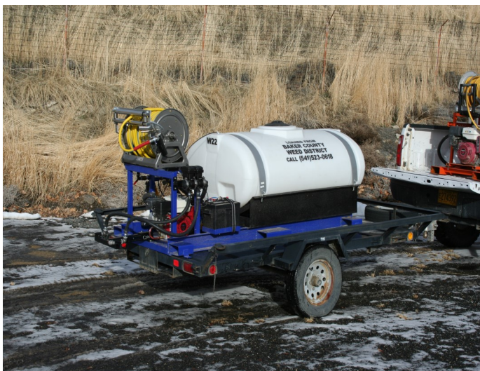
25 gal Sprayer on trailer — 40 ft boomless spray width 6 acres treated per load — 300 ft handgun/reel $40.00 per day
