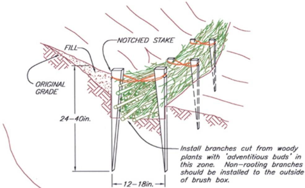
Brush box at the toe of a slumping or raveling slope.
