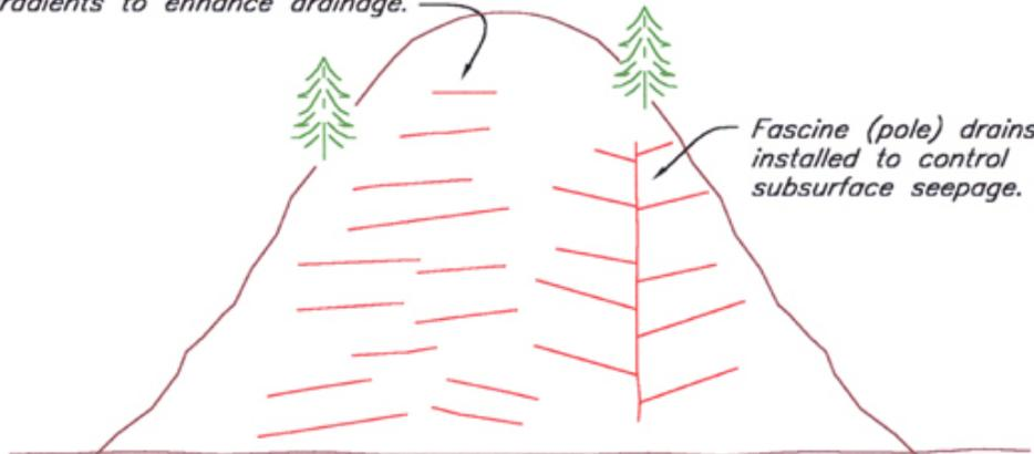
Fascine (pole) drains installed to control subsurface seepage.
