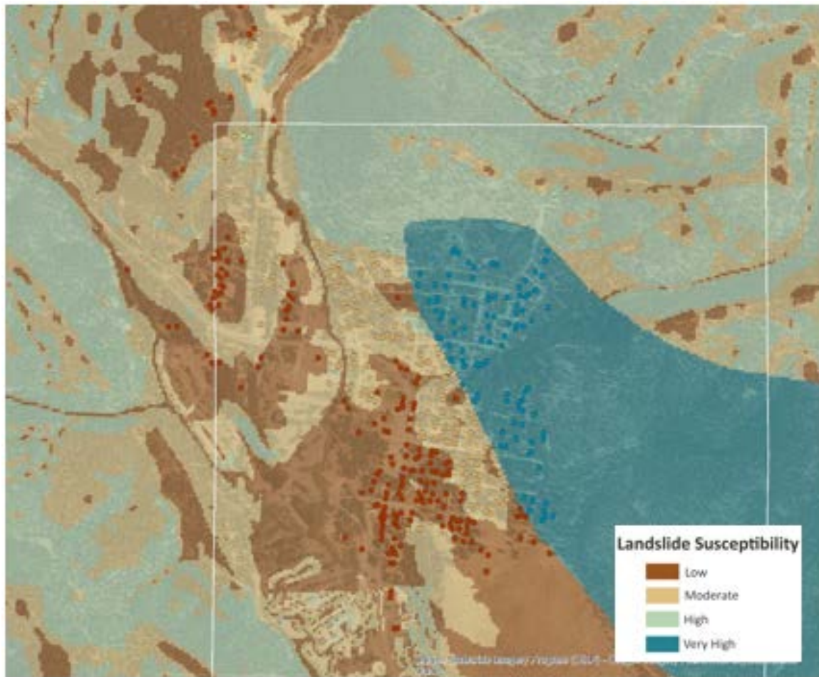
Figure 11. Landslide susceptibility areas and building exposure example in the City of Sumpter
